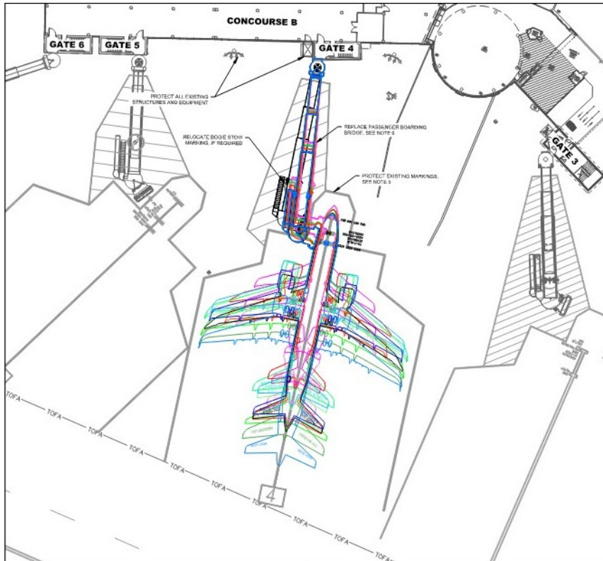
PASSENGER BOARDING BRIDGE - AIRCRAFT COMPATABILITY TABLE
